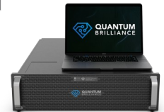
Quantum Brilliance NV diamond quantum machine ("a few" qubits)
