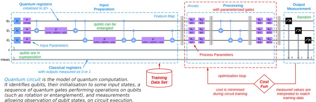
Quantum circuits are static - new data requires new circuit. However, it is possible to create "variational" circuits, which are templates with parametrised gates, e.g. P, Ry and Rz varying degrees of rotation, which can be optimised using some ML algorithm.
