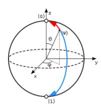
When measured, the qubit state "collapses" into one of the basis states |0> and |1> resulting in a value of "0" or "1" to be observed
